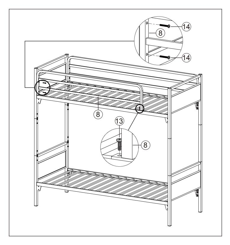
• ATTACH SHORT GUARD RAIL (8) ONTO UPPER BED USING ALLEN BOLT (13) AND ALLEN BOLT (14).
