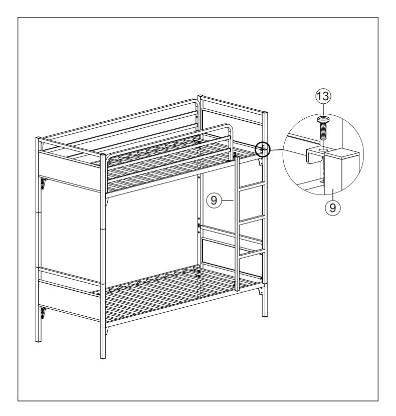
• ATTACH LADDER ONTO BUNK BED USING ALLEN BOLT (13).
