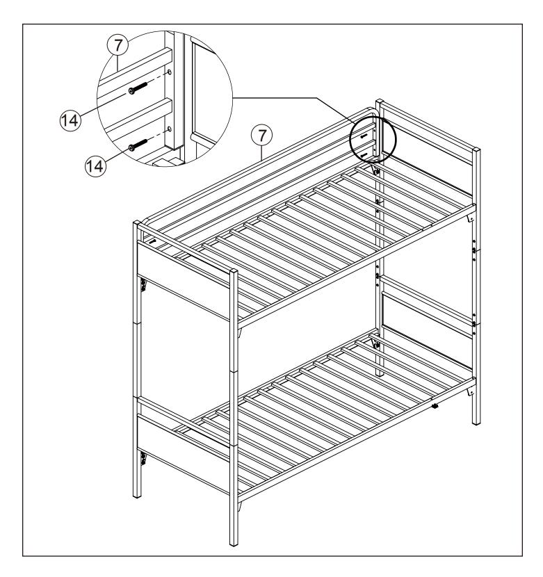
• ATTACH LONG GUARD RAIL (7) ONTO UPPER BED USING ALLEN BOLT (N).
