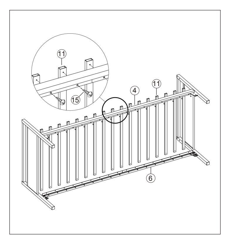
• ATTACH SLATS (11) TO FRONT RAIL (4) AND BACK RAIL (6) USING SCREWS (15).
