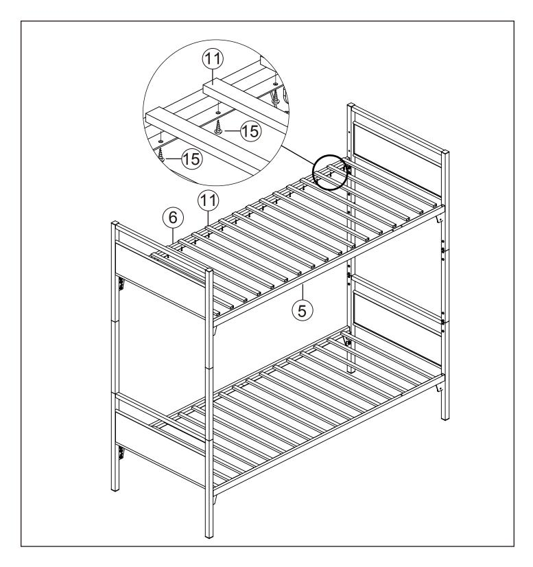
• ATTACH SLAT (11) TO FRONT RAIL (5) AND BACK RAIL (6) USING SCREW (15).
