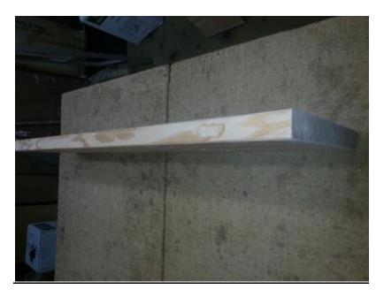
Lay the 2" x 12" x 44" On Edge, As Shown In The Image. Place the 2" x 12 x 19-1/2" Top Shelf On Top Of The 2" x 12" x 44". That Is On Edge. Drill The Screws In To The Wood, Nice And Tight.
